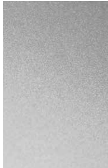
BEAD BLASTED – EVEN AND MATTE SURFACE
